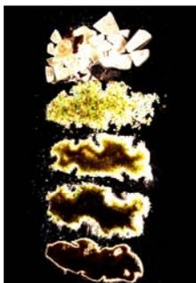
Both recycled container and flat glass have been used in shot blasting applications. The application is not colour sensitive so mixed colour recycled container glass can be used. The standard screening and metal removal techniques are sufficient to achieve the quality of material required for this application, however fine size reduction and classification are needed.
