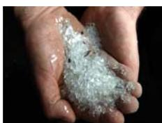
Glass below 5mm represents no special hazards; at this particle size no sharp edges are evident, although, as with other shot blast media, gloves are recommended when handling.
